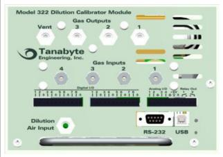
Number of Gas Outputs: 4 Outputs 1/4" Tube OD Gas Outputs Fittings Size: Number of Gas Inputs: 4 Inputs Gas Input Fittings Size: 1/8" Tube OD Number of Analog Outputs: 4 Outputs Number of Digital I/Os: 16 I/Os Number of Air Inputs: 1 Input 1/4" Tube OD Air Input Fitting Size:
